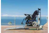
Secure the wheelchair using the supplied straps and store the telescopic ramps in the appropriate housings.
