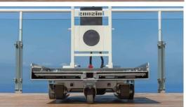
When not working on stairs with the tracks, the three wheels with which Domino People is equipped always rest on the ground to facilitate movement from one step to another.
