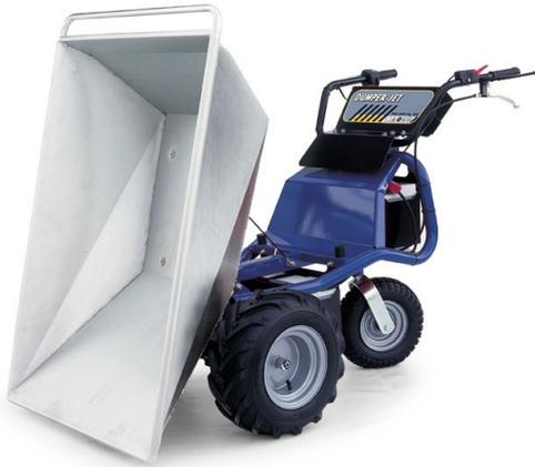
The Dumper Jet is an Electric wheelbarrow designed to work with loads of up to 400Kg. The strong frame is made of steel and powder coated with exterior paint. The right balance between the load and the wheels, gives the user confidence, and increased its manoeuvrability.
