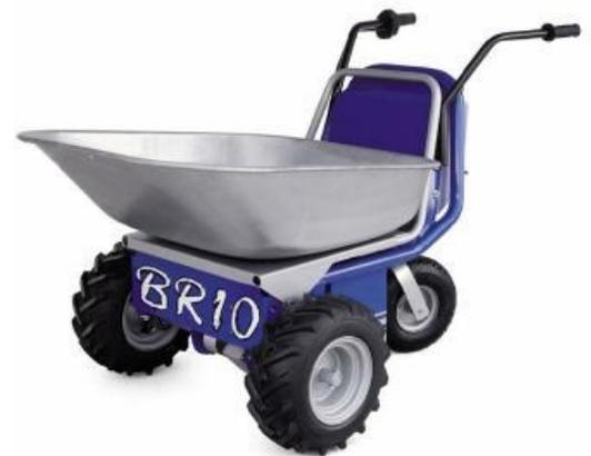
The 300W motor has an electromagnetic brake that stops the Brio accidentally slipping while on ramps up to 30% with a full load. The gears in oil bath avoid any kind of maintenance and the machine can be cleaned easily without causing short circuits thanks to the controller and the well cabled wires kept in an hermetic ambient.
