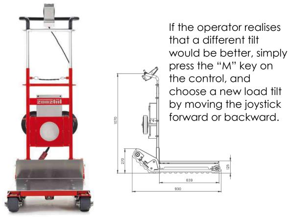
DOMINO Automatic will store the new reference for the subsequent stair ramps, making transport safer.
